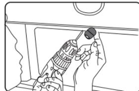
6. Fasten the second screw and securely tighten both screws.
