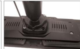
Fig. 4: OEM replacement mount
